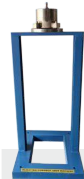
Bursting Chamber Unit Machine. (Ref. Standard: ASTM D 751-95.) Made of SS-304 Machining Process
